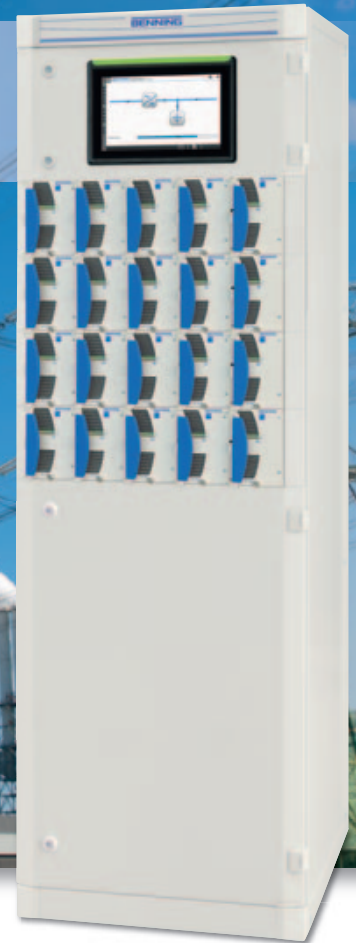
Figure 3: DC power supply systems of 60 kW, based on 4 rectifier rack units, each with 5 output modules (max. 15000 W output power).
