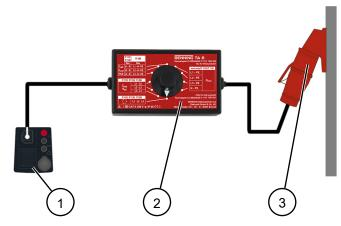
Figure 3: Connecting the BENNING TA 6
