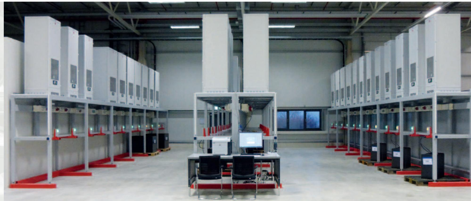
In March 2015 the battery test facility with 50 stations went into operation.
