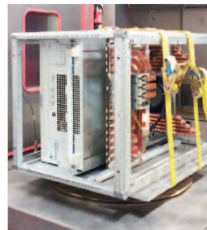
Component testing on a shaker in the BENNING test laboratory
