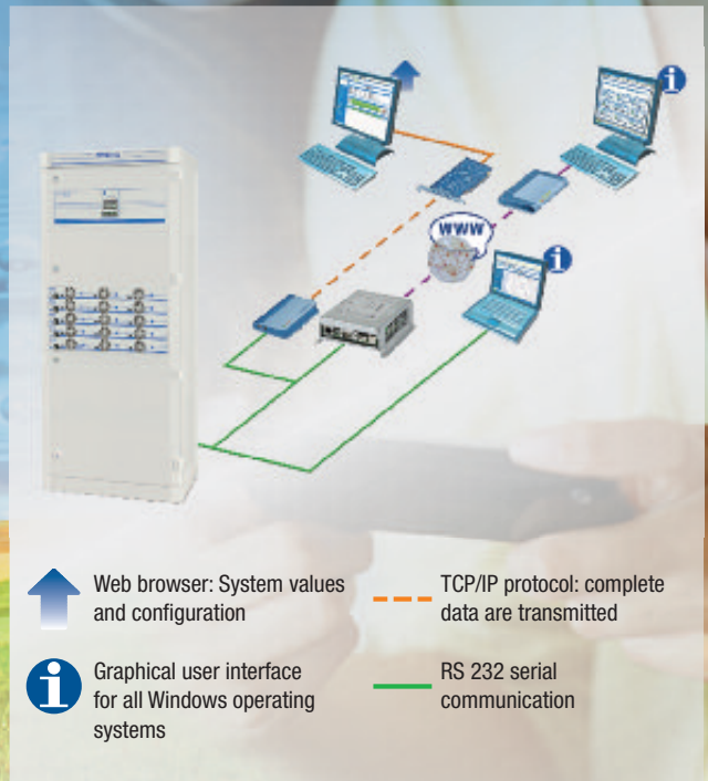
Fig. 9: MCU 2500 remote monitoring system
