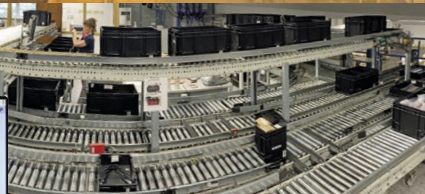
Automated container feed and commissioning area in "AKL" (= automated small-parts store)
