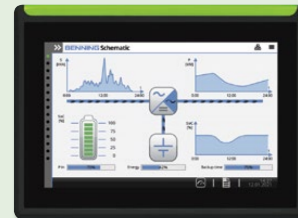
The MCU (monitoring & control unit), with its diversity of supported protocols and interfaces, makes it possible to connect the system to EMSs of the widest range of software manufacturers. The system controller (MCU 3000) integrated into the power supply system cabinet door comes with a 10.4 inch touch display.
