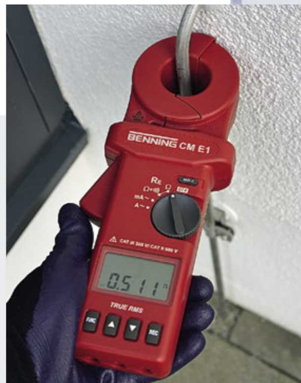
Testing a lightning conductor system using the BENNING CM E1: grip the earth conductor with the clamp, take the reading and you're done.
