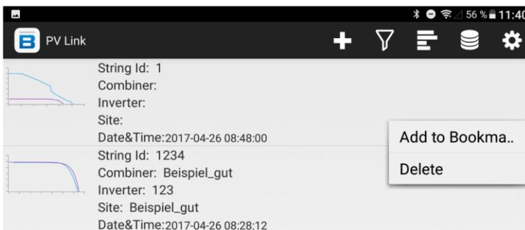
Via the start screen, you can read new measurement data from the BENNING PV 2, filter or sort measurement data, delete all existing measurement data and make various settings.
