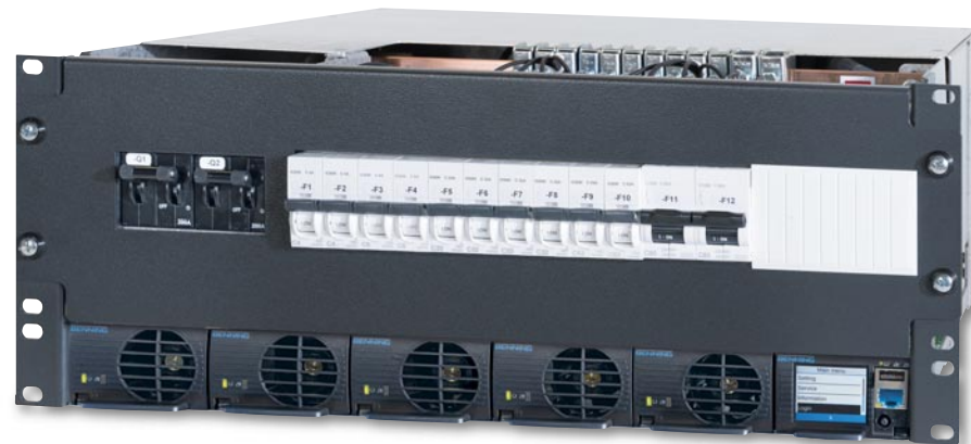
Fig. 6: SLIMLINE system 48 V / 10 kW with a SLIMLINE controller, as well as battery and consumer distribution. Power ratings of 2 – 34 kW can be achieved by scaling the rectifiers and adapting the distribution.
