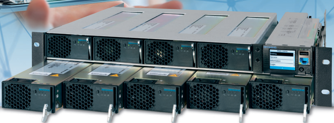
Fig. 3: The 19" 1H carrier can accommodate either four 48 V and 3000 W rectifier modules combined with a controller or five rectifier modules.
