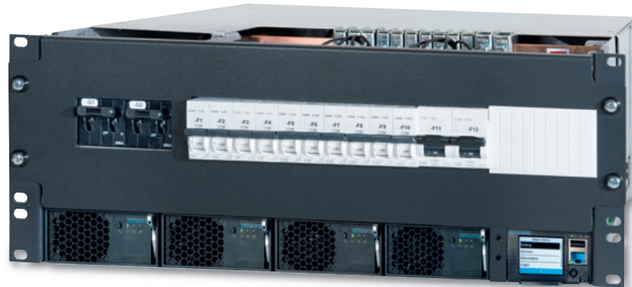
Fig. 6: SLIMLINE system 48 V / 12 kW with a controller, as well as battery and consumer distribution. Power ratings of 3 – 27 kW can be achieved by scaling the rectifiers and adapting the distribution.
