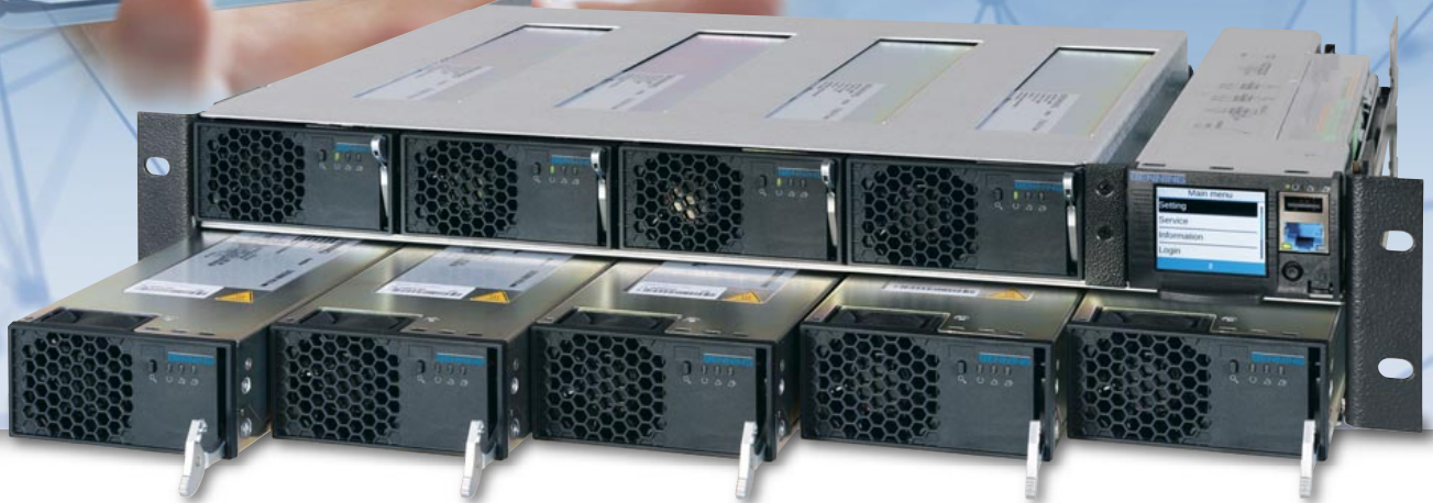
Fig. 3: The 19" 1H carrier can accommodate either four 48 V and 3000 W rectifier modules combined with a controller or five rectifier modules.
