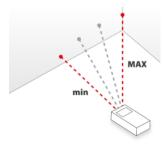
Figure 4: Length measurement (continuous measurement, exemplary)
