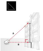
Figure 7: Indirect length calculation (exemplary)
