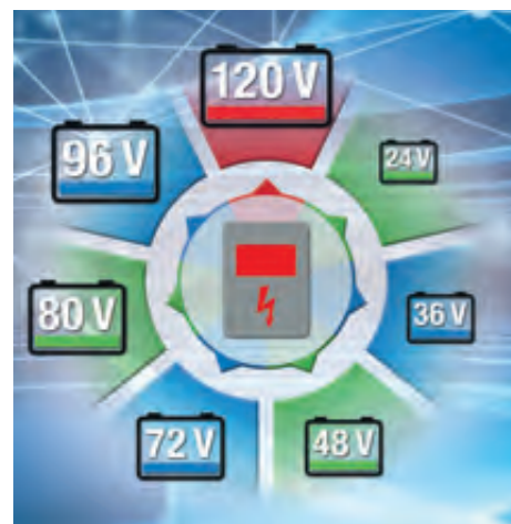
Batteries of different voltages are assigned to different NBS groups. The BELATRON chargers with the multivoltage option automatically assign themselves to the correct NBS Dynamic group.
