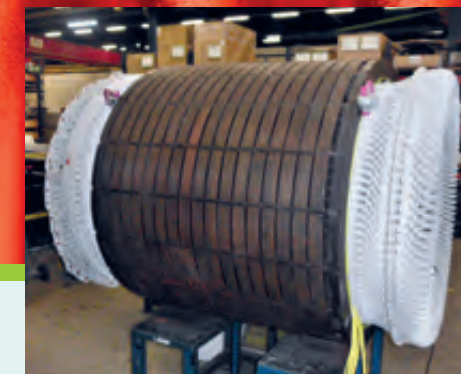
Newly wound stator before impregnation
