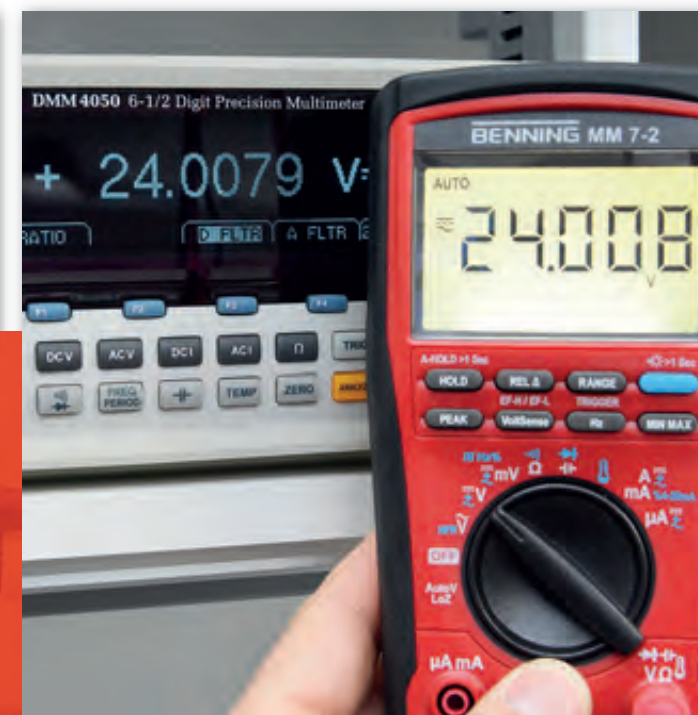
0.03% basic volts DC accuracy for precise readings and demanding metrology tasks (comparative measurement in laboratory with a calibrated precision laboratory multimeter)
