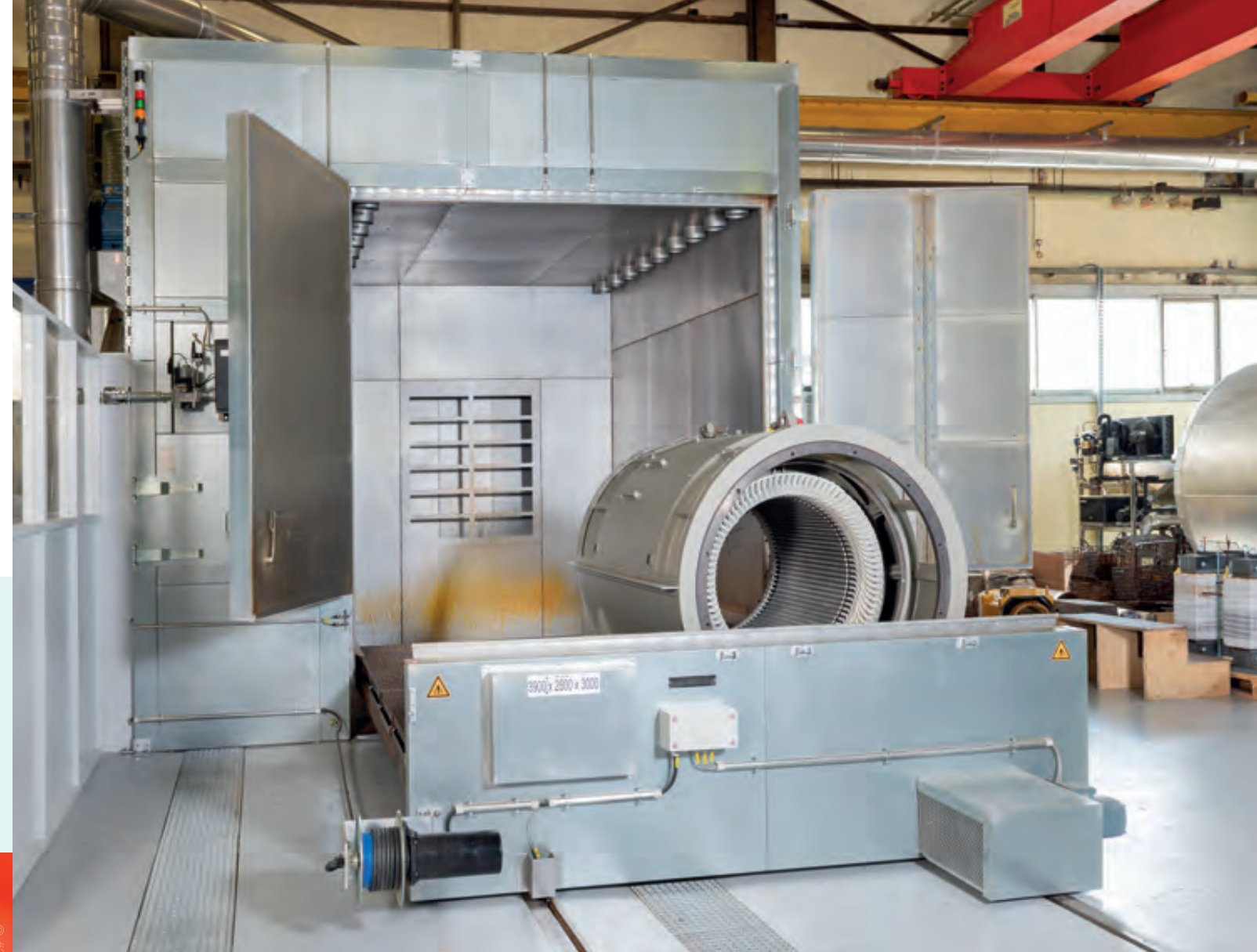
A finished component is moved out of the drying oven
