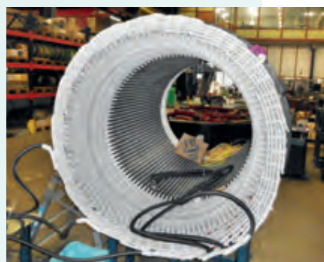
Newly wound motor (above) after and (below) before impregnation
