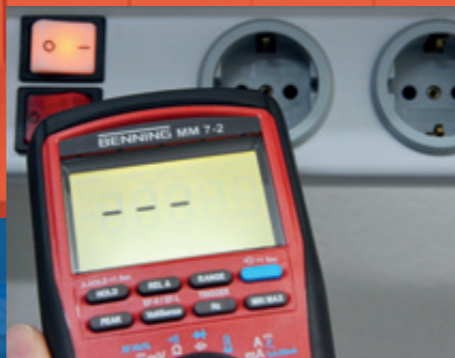
(at right) Contactless voltage detection. This also means that line breaks – such as in extension cables, for example – can be readily traced
