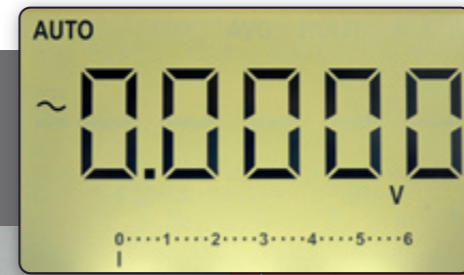
High-contrast display with characters 15 mm high, and a 30-segment bar graph
