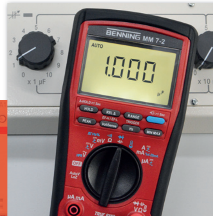
0.01 nF to 10 mF capacity measurement range
