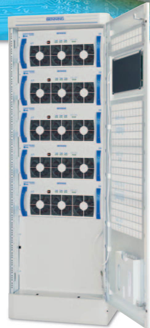
ENERTRONIC modular SE with 20 kVA power modules. Output power 80 kVA (n+1)
