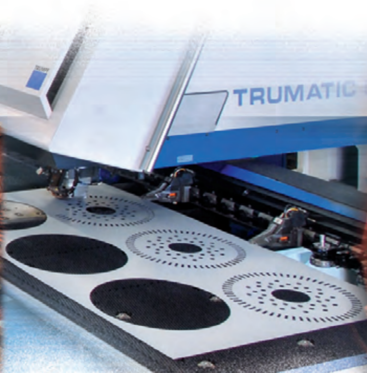
CNC stamping of laminations
