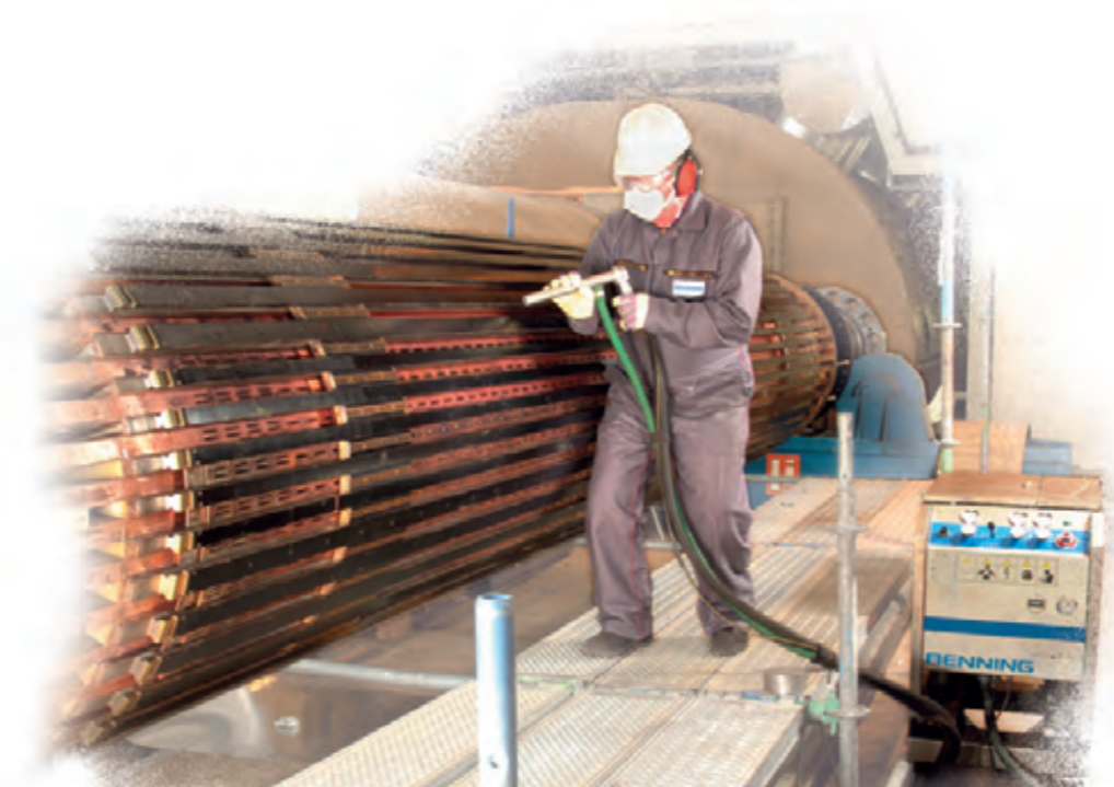
Dry ice cleaning of a generator rotor on job site
