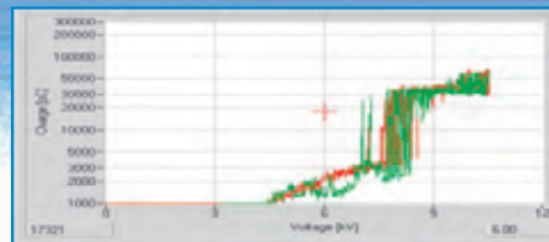
Partial discharge test of an electrical machine in critical condition
