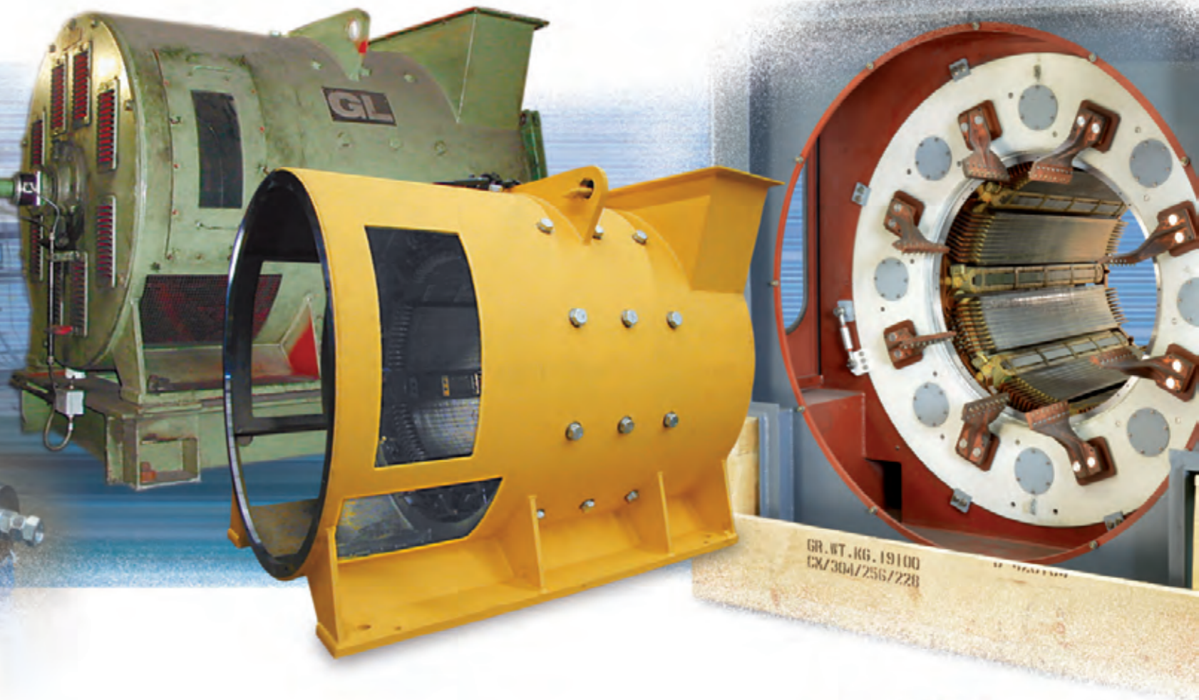
Original machine and reproduction: DC motor, 780 kW, 500/100/1500 rpm
